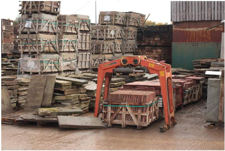
Top image: Reclaimed structural timber, stacked and aired for drying in the yard . Lower image: Mechanical lifting facilities for palleted reclaimed tiles. Previous page: Overall view of yard at Cheshire Reclamation.
