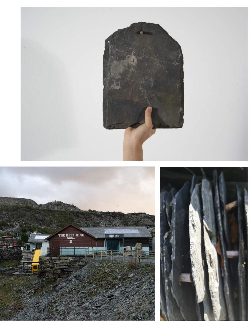
Top image: gray-blue slate roofing tile with original wooden peg Bottom left: Llechwedd Slate Cavern - quarry and mine attraction Bottom right: Stacking of slates from West Wales Reclamation
