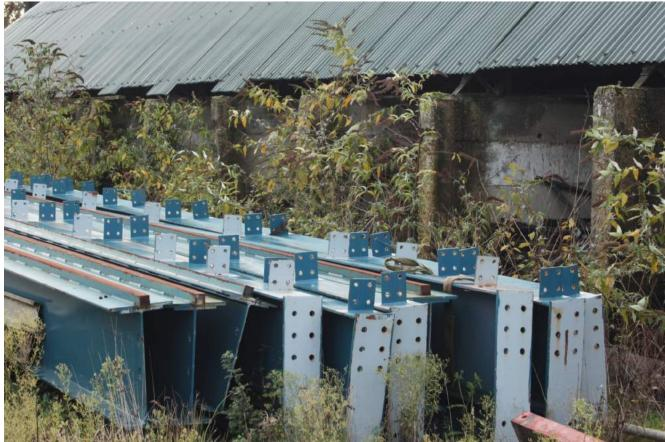
Previous Page Image; Workshop at Portal Power, Top Image; Elements of Portal Frame being stored at Portal Power, including galvanised 'cleat' pre- attached to rafter. Lower Image; Elements of Portal Frame being stored at Portal Power as kit of parts.
