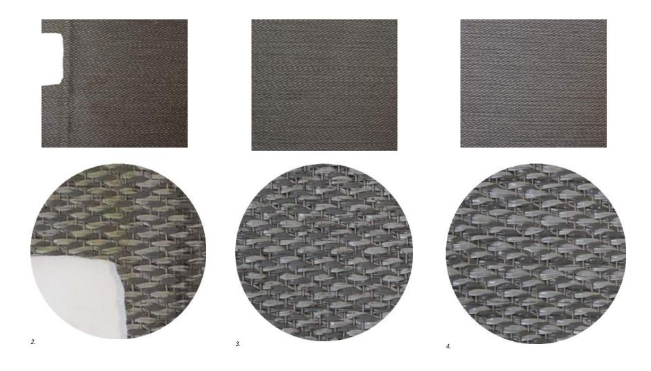
1. High-end reused wood 2. Damaged Carpet tile 3. Carpettile to be reused 4. New Carpet tile
