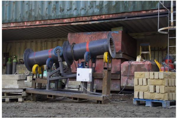
Top image: Stones laid out ready for London paving at Abacus Stone Sales. Lower Image: Stone tumbling machine for artificial weathering of new stone.
